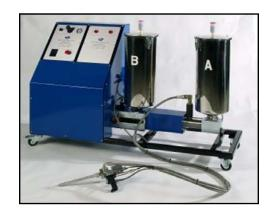
Metering Pumps: Single acting positive displacement.
