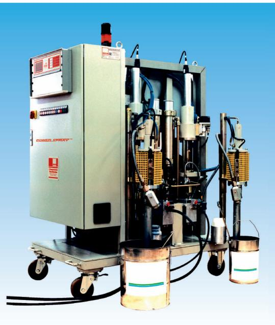
**PowerSpray** Servo hydraulic actuated High Pressure Metering system for corrosion protection
